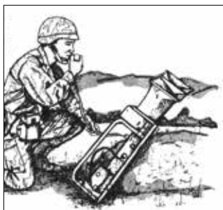
The 250-watt ‘man-packed’ AN/UIH-6 loudspeaker was taken on and off like a backpack, and had an average audible range of a quarter to half a mile.
