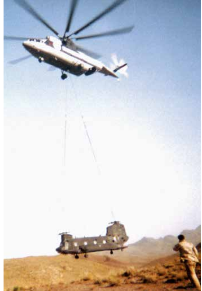
The Mi-26 lifts 476 from its crash site. Once it left, the maintenance crew followed in another Chinook.
