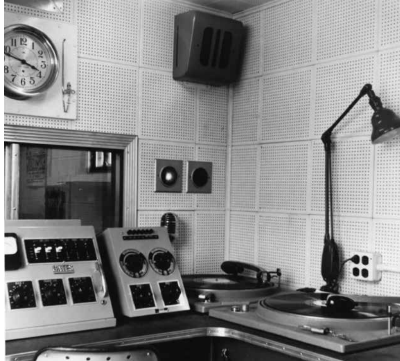
Depicted here is the standard studio set-up in the MRBC’s 35-foot transmitter van (AN/MRT-5), including a mixing board with two master mix faders, a 1/4” tape recorder, and a 33 1/3 RPM turntable. Except for the tape recorder, all equipment was made by Gates Radio Company, Quincy, Illinois.
