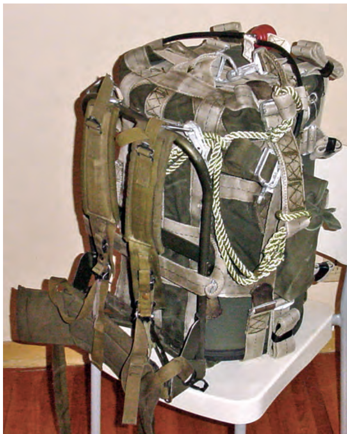
In 1962, Special Forces was assigned to deliver and detonate the B-54 Special Atomic Demolition Muniton (SADM) shown rigged for airdrop.
