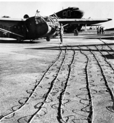
Waco C6-4A glider tow ropes had to be laid out very carefully to avoid tangling during takeoff. The sturdy ropes served as a literal lifeline until gliders were aloft and able to maintain altitude on their own.
