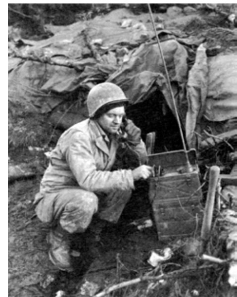
The workhorse radio of the frontline troops was the SCR-300 walkie-talkie. At 40 pounds, the SCR-300 was man-portable and had a range of up to 25 miles.
