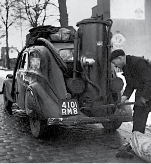
Gasoline shortages in Occupied France during WWII forced the French to be creative. This late 1930s French Renault sedan has a charcoal burner installed in the trunk.
