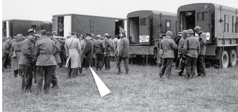
The mobile radio station at Fort Riley: During the graduation of PSYWAR Class #1 the mobile radio station was set up for visiting dignitaries. This was the prototype system. It would take a few months to produce the systems for the 1st RB&L in Korea. The two vans on the left are production studios; on the right are the radio transmitter and receiver, each mounted in a truck shelter. In the center of the photo are BG McClure, the Chief of PSYWAR (indicated by arrow) and COL Greene, the Chief of PSYWAR for FEC.
