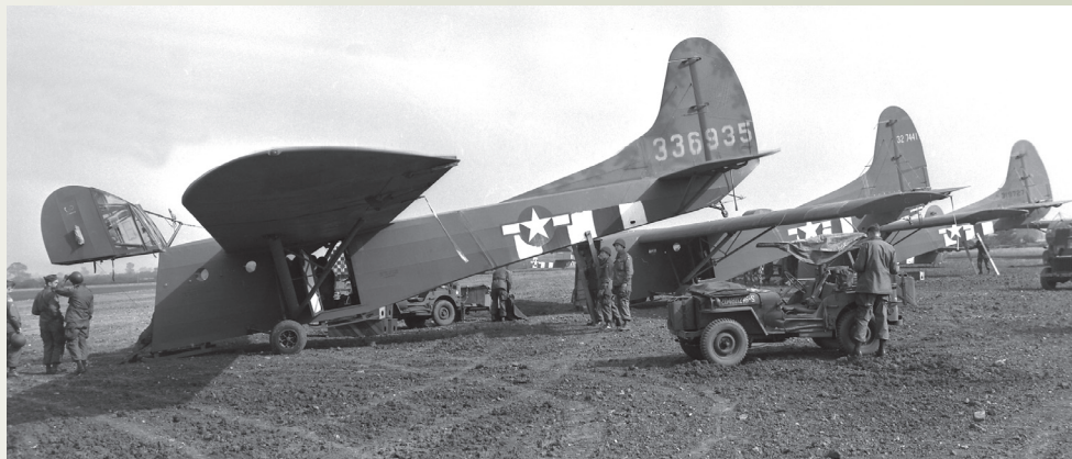
CG-4A "WACO" gliders ready for loading. Notice the pilot's compartment in the raised nose section and the wooden supports used to elevate the tail to keep the cargo compartment on the ground. This technique made it easier to load bulky supplies and equipment into the glider.
