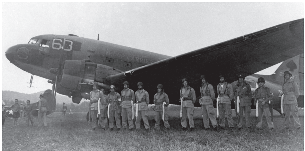
The C-47 "Sky Train" was the workhorse of the USAAF in every theater of operations. It performed a variety of missions from transporting supplies and equipment to dropping paratroopers and towing gliders. Each paratrooper pictured is equipped with a lowering line for use in the event of a tree landing.
