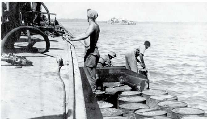
At Kyaukpyu, P-564 had to be refueled from 55-gallon drums transported from shore in amphibious DUKW "ducks" because destroyed port facilities prevented the Air-Sea Rescue Boats from docking.
