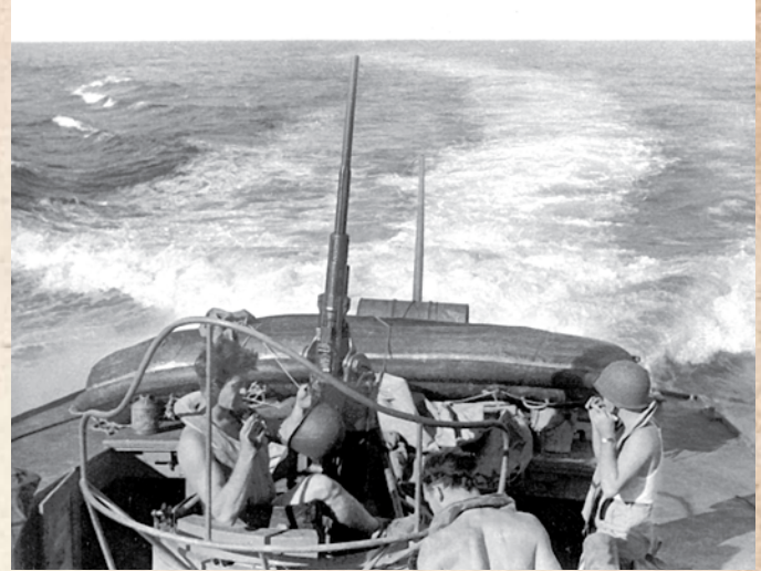
P-564's main armament was a 20 mm Oerlikon cannon, mounted at the stern. Operational equipment, such as the LCR in this photograph, was also stowed there.
