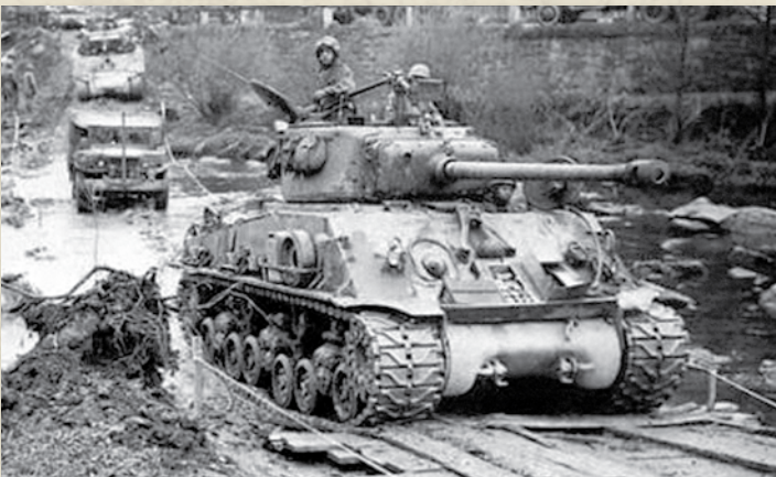
M4A3E8. Nicknamed the "Easy Eight", this tank was the improved version of WWII's M4 Sherman. Armed with a 76 mm main gun, it was also replaced by the M46 Patton.
