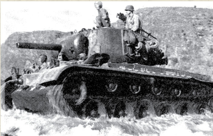
M45 Howitzer Tank. This was a 105 mm howitzer mounted in the turret and hull of an M26 Pershing chassis. It was found in the assault gun platoon of the Medium Tank Battalion.
