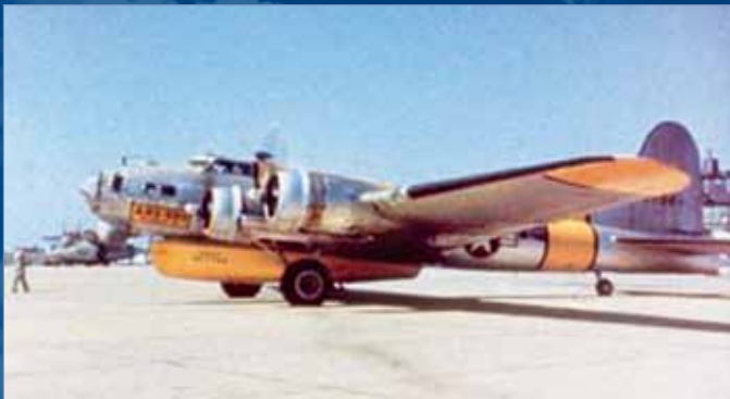
The SB-17 Flying Fortress carried an air droppable life boat under its fuselage.
