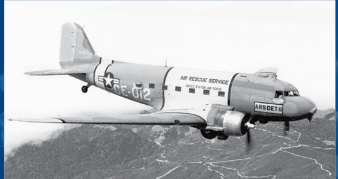
The SC-47 Skytrain carried rubber life rafts which were airdropped to airmen downed over water.
