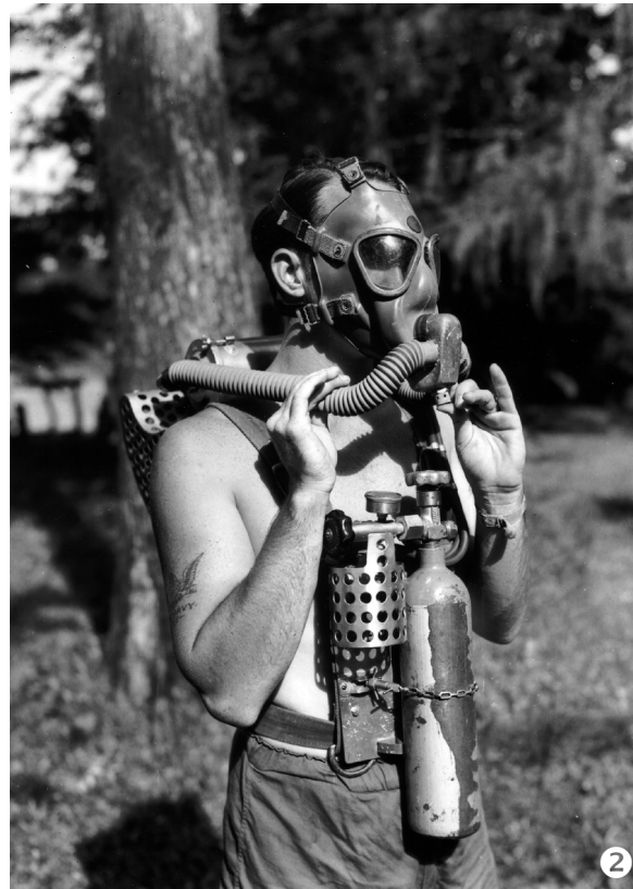
❸ Lt. Fred Wadley wearing LARU Model 10 (LARU)(out-of-water)-late 1944. Extended swim fins, depth gauge, waterproof watch, m3 Trench Knife, Double-gimbaled Compass Bracket (Army Engineer Compass), OD Longjohns, Speaking Diaphragm.
