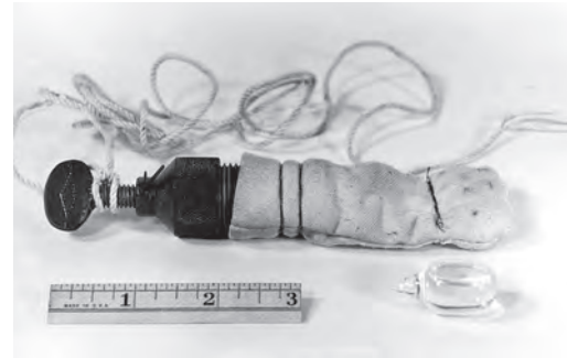
The OSS 'Dog Drag' was designed to confuse tracking dogs. When crushed, the glass vial emitted a noxious odor.
