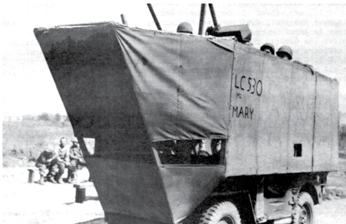
Before live firing the Landing Craft MCM .50 cal Browning M2 machine guns from the sea, the 38th ID infantrymen were oriented to the height and swaying motion using this Jeep mock-up.
