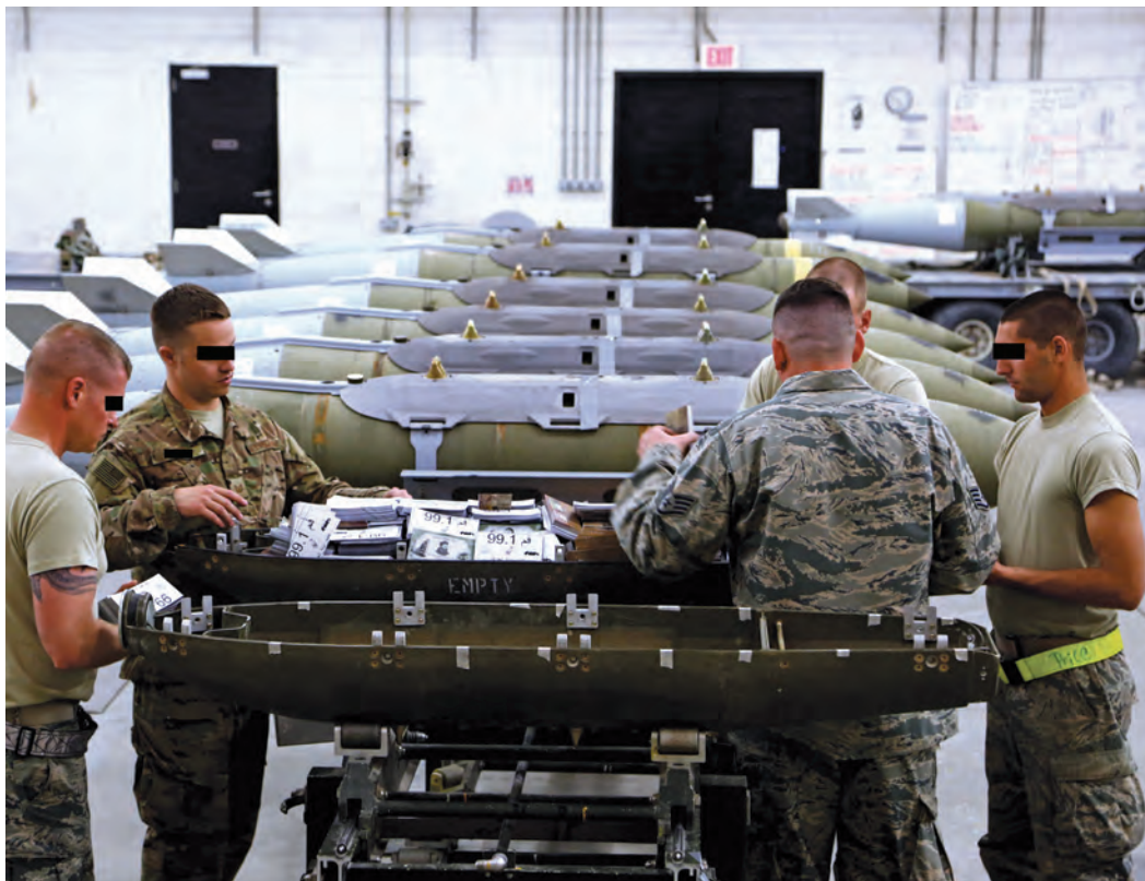
U.S. Army and Air Force personnel load a 750-pound M129 E2 bomb canister with MISTF-C leaflets to be dropped by B-52 Stratofortress aircraft. After the M129 is dropped, a time fuse detonates the primer cord between the bomb's two sections, blowing it open and releasing its contents on target audiences within the Combined Joint Operations Area (CJOA). 7
