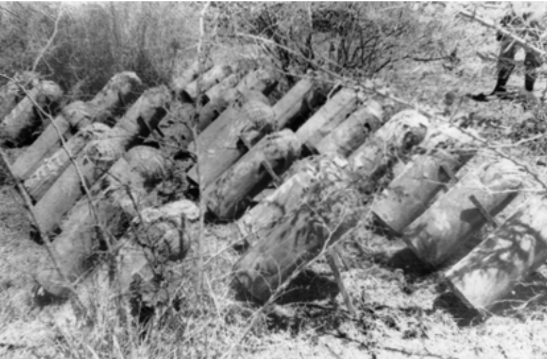
Field of artilleria sin cañon discovered outside the cuartel. These were made from sheet metal stove pipe.
