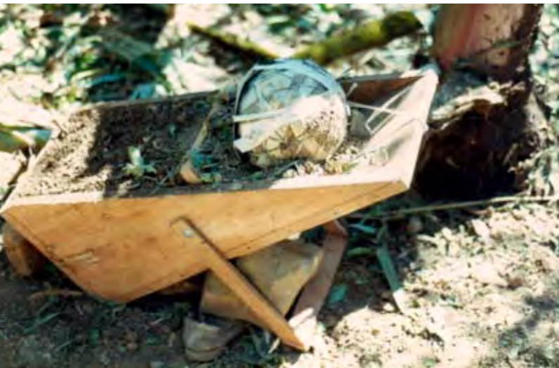
A close-up of artilleria sin cañon or rampas showing wooden launchers with adjustable legs to set elevation. Earth was tamped against the backplate.
