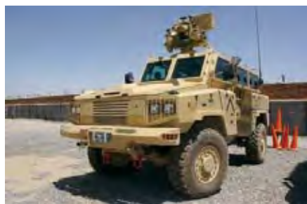
The RG-31 Nyala, made by the South African firm of Land Systems OMC, is a multi-purpose mine-protected vehicle. It features a "V"-shaped hull and has high ground clearance.
