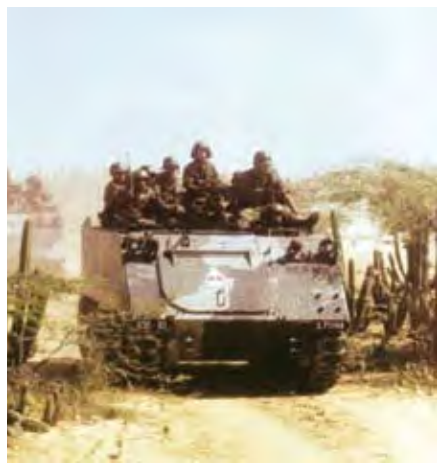
The M-113 is a U.S.-produced armored personal carrier and is in widespread use worldwide, seeing use in some forty-four militaries. It can carry eleven personnel and two crewmembers. Although it can be armed with a number of weapon systems, the most common are a heavy machine-gun or a grenade launcher.
