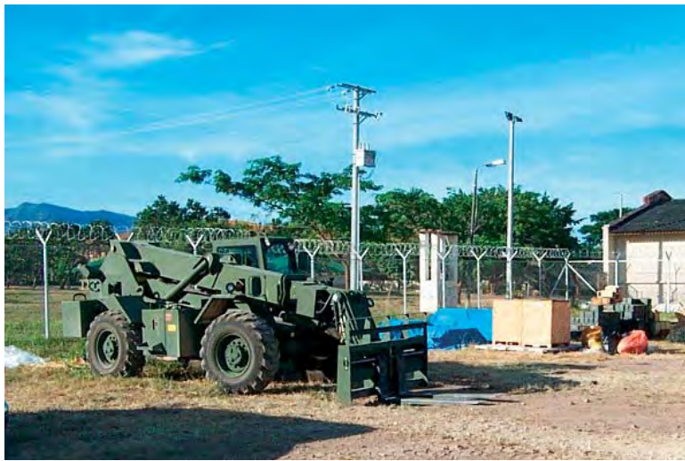
"Atlas," the rough-terrain forklift, provided the ammunition handling capability at the ASP in Tolemaida.
