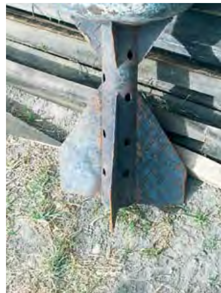
Non-slip pattern sheet iron (commonly used to make custom step-ups on U.S. trucks) fins for a bomba barbacoa.
