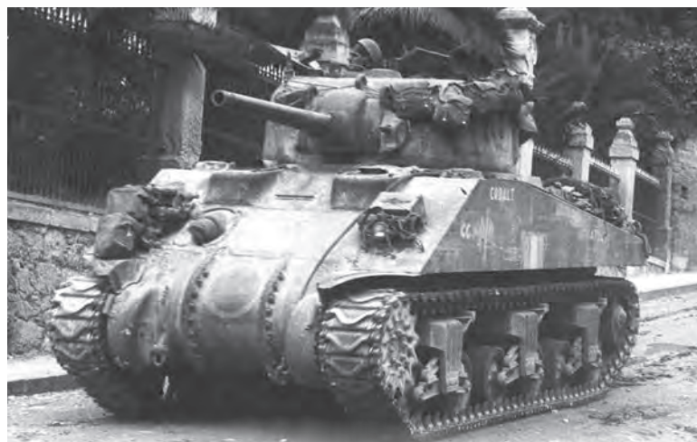
The M4, more popularly known as the Sherman, was the standard U.S. Army medium-tank of the war. It was produced in large numbers and was easy to maintain, but was out-classed both in armor and armament by many German tanks.
