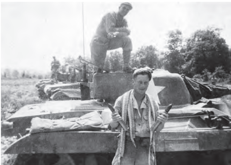
The M22's 37mm main gun fired the small shell held in the crewman's hand. Such shells would have had little effect on German armor.
