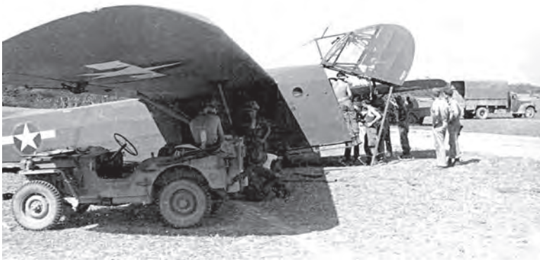
The CG-4A Waco glider was the basic U.S. Army glider of WWII. This example, being loaded by OSS Detachment 101 in Burma, has the nose flipped open to allow easier access.
