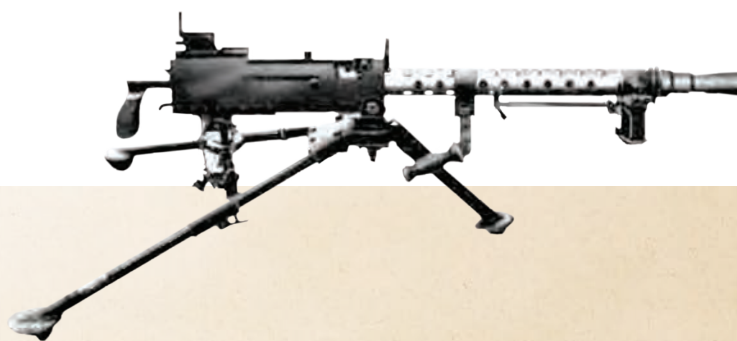
The WWII-era M-1919A6 light machinegun was capable of firing 600 rounds of .30 cal ammunition per minute.
