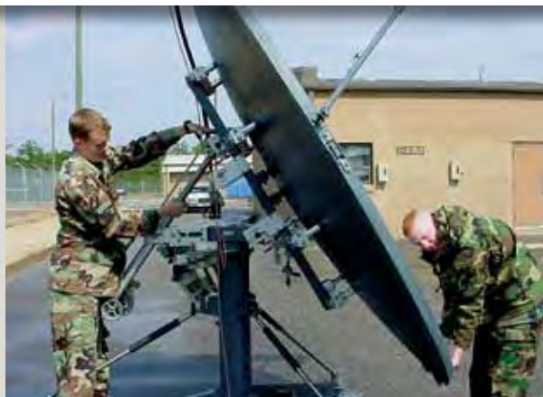
Soldiers of the 112th Signal Battalion erect a Down-sized Deployable Satellite Terminal (DDST). The 112th's capability to transmit and receive voice and data globally via satellite communications systems extends the reach of ARSOF units around the world.
