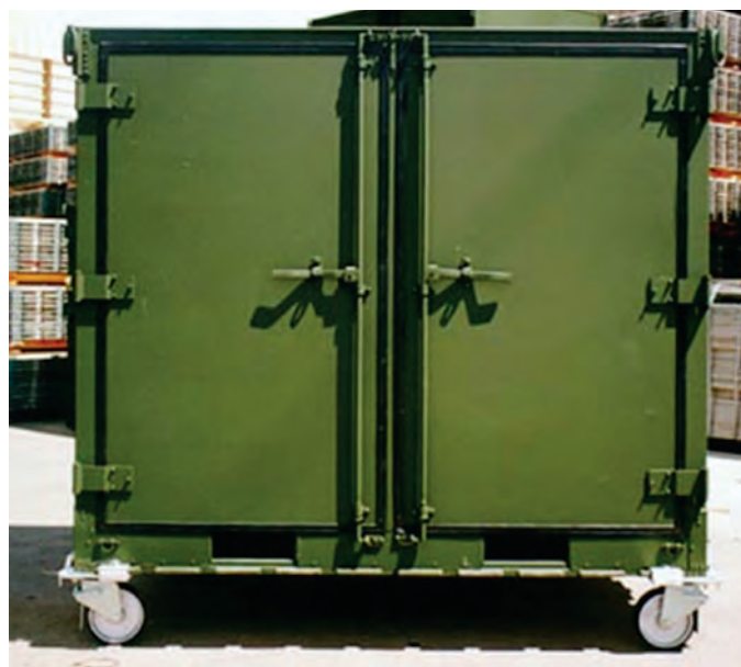
An ISU-90 container (90" x 88" x 104"). The SORT was designed so that all its equipment could be loaded into three of these units for shipment on Air Force cargo aircraft.
