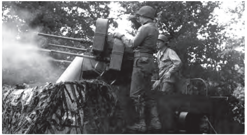
With the German Air Force threat reduced to nothing, anti-aircraft "quad 50s" were used as ground support weapons. The four .50 caliber machineguns could send a hail of bullets at the enemy. (Center for Military History)
