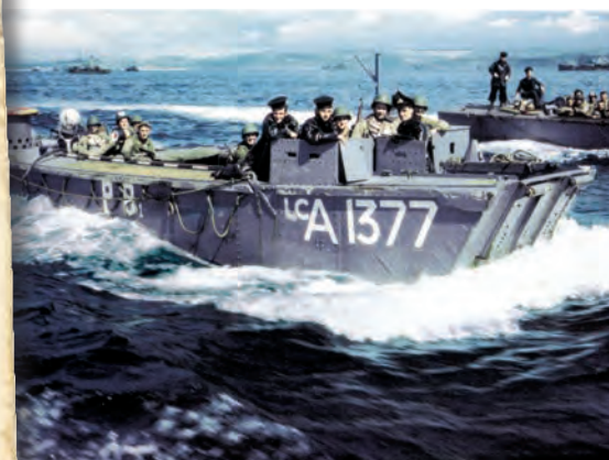
5th Rangers riding British Landing Craft Assault (LCA) 1377 to the HMS Prince Baudouin in preparation for the D-Day landings. The Rangers preferred the LCA because they had benches to sit on, speed, and an armored bow for protection. In the center of the photo is Major Sullivan, to his left Royal Navy Sub-Lieutenant Ernest "Joe" Pallent, commander of the British landing flotilla, and Captain John C. Raaen, Jr., the Headquarters Company Commander (far right). (National Archives)
