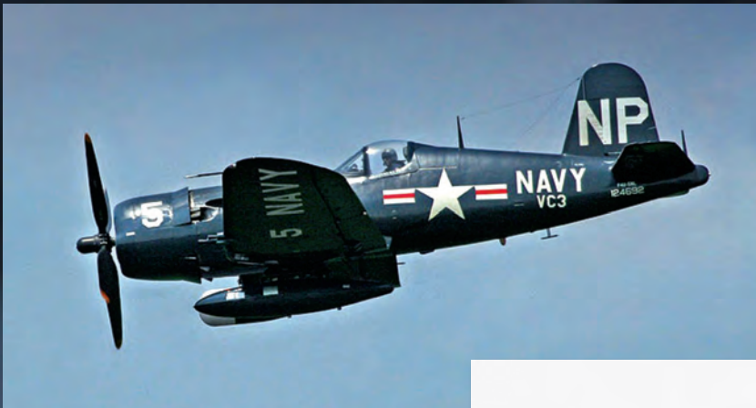
An F4U-5N all-weather, radar-equipped Corsair like that flown by LT Bordelon in 1953.
