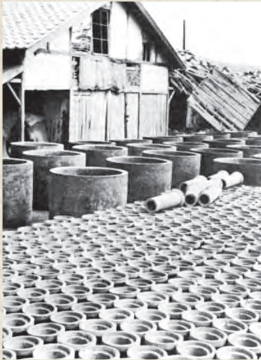
Cement donated by UNCACK was used to make culverts and well casings in July 1952. As the war grew static, UNCACK's mission shifted to that of helping rebuild the South Korean economy.
