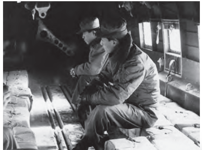
Korean military "door kickers standing-by" leaflet "bricks" containing pull-ring mechanical fuse igniters.
