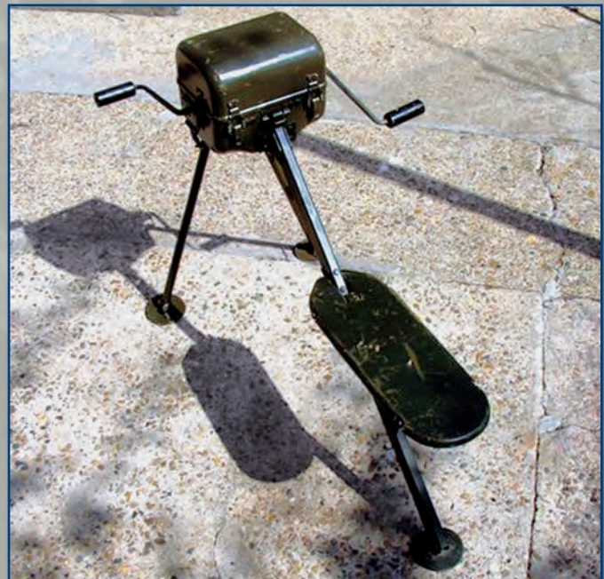
GN-58 hand-cranked generator for the AN/GRC-9.
