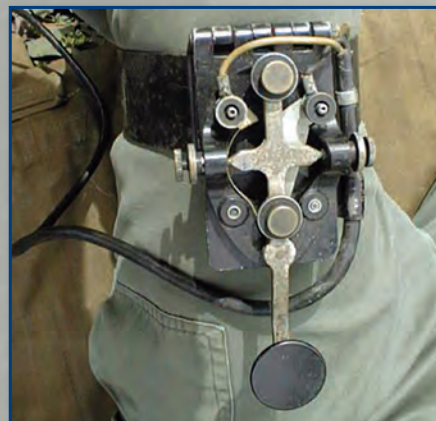
CW, or Morse Code key for the AN/GRC-9 radio.
